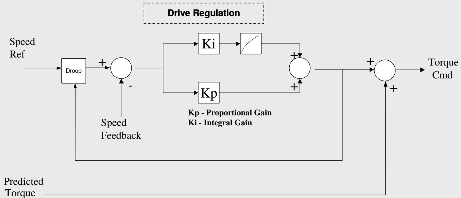
The above droop regulator is excellent for an application where low nip pressure “Soft Nip” exists between felts.
